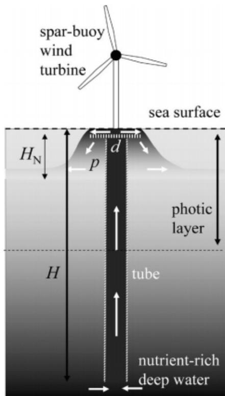
Fig. 1. – Schematic of the spar-buoy turbine upwelling device illustrating its essential (not to scale) parts. Labels indicate the negative buoyant plume ( $p$ ), the pipe's bottom depth ( $H$ ), neutral height ( $H_N$ ), and diffuser platform ( $d$ ). White arrows indicate water flow and the grey shade qualitatively indicates nutrient concentration.
